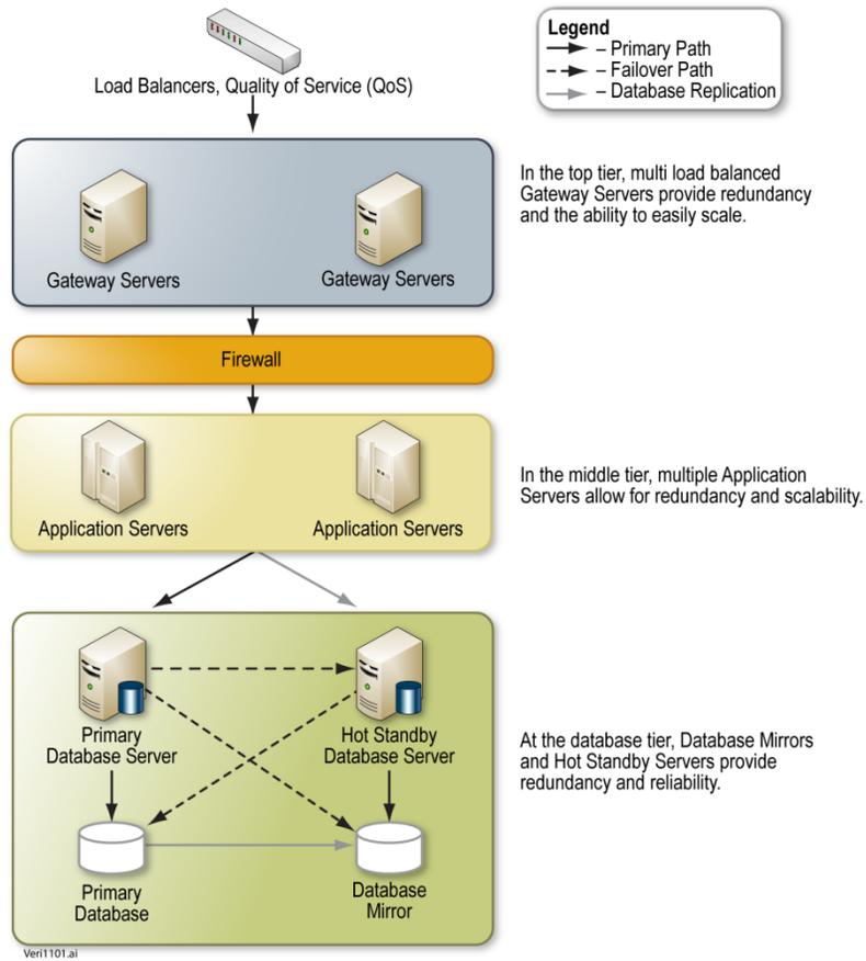
**Figure 24-1: SRS Architecture.** Verisign's SRS is hierarchically designed to meet the forecasted registration volume of the .ABC gTLD, and it can be scaled to meet future registration volume increases.
