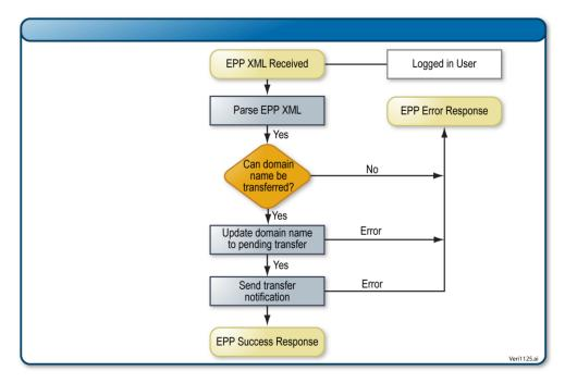
**Figure 27-5: Transfer Request Process**
