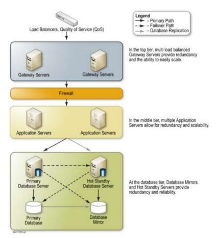
**Figure 24-1: SRS Architecture.** Verisign's SRS is hierarchically designed to meet the forecasted registration volume of the .LIVE gTLD, and it can be scaled to meet future registration volume increases.
