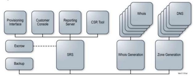
**Figure 24-4: Technical Overview.** Verisign's SRS provides the registrar-facing component of the system establishing the zone file needed to enable DNS and Whois services.
