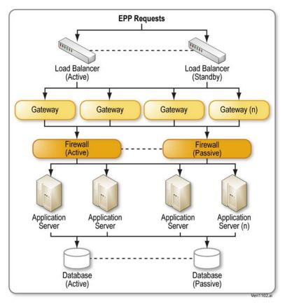
**Attachment 24-2: Built-in SRS Redundancy.** *Verisign's SRS system is built upon multiple layers of redundancy to ensure the system remains highly available.*
