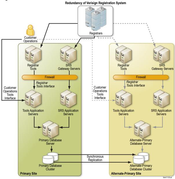
SRS Network Diagram. Verisign's fully redundant SRS design and geographically separated data centers help ensure service level availability requirements are met.
