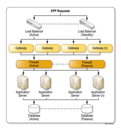
**Built-in SRS Redundancy.** Verisign's SRS system is built upon multiple layers of redundancy to ensure the system remains highly available.
