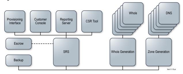
**Technical Overview.** Verisign's SRS provides the registrar-facing component of the system establishing the zone file needed to enable DNS and Whois services.
